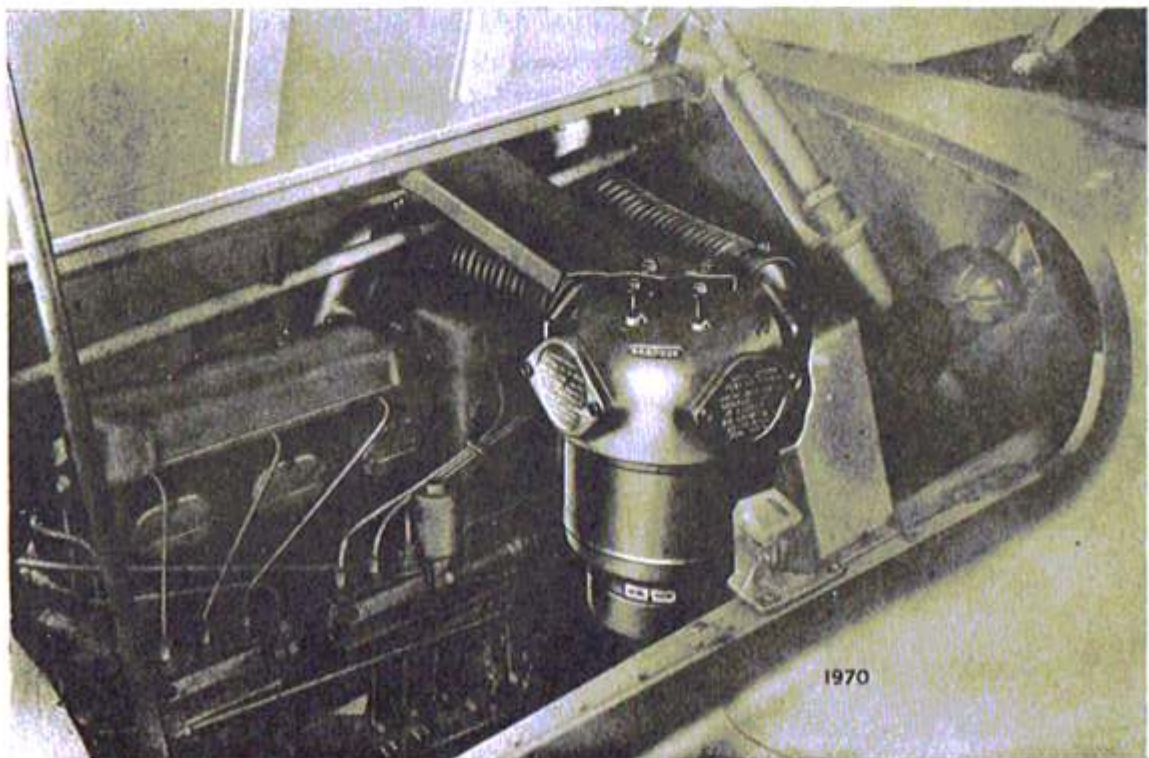
Fig. 39. UNDER-BONNET INSTALLATION OF UNIVERSAL OIL BATH TYPE AIR FILTER ON A DOUBLE-DECK PASSENGER VEHICLE
